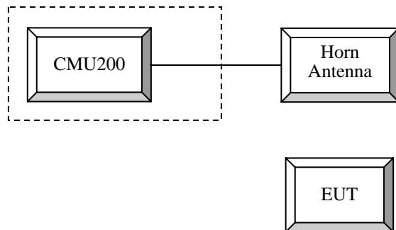
**Block Diagram of Test Setup**
