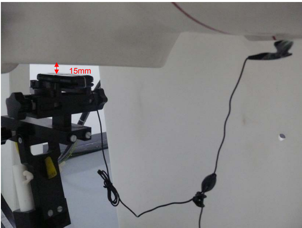
Picture 13: Body with earphone, The EUT display towards ground, the distance from handset to the bottom of the Phantom is 15mm (Close)
