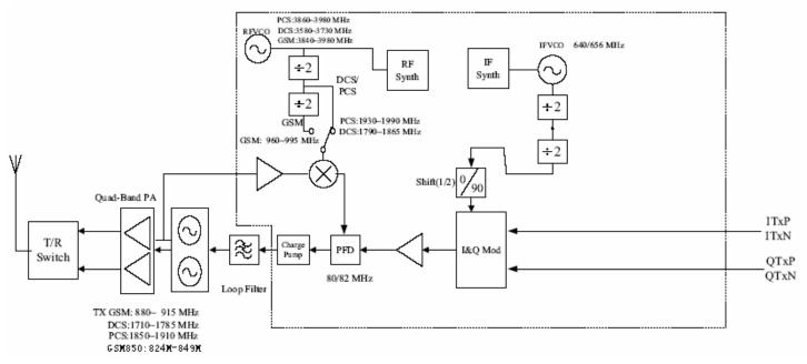
The frequency ranges of the synthesizer for TX mode are TX mode GSM850 1813M -1868M PCS 2035M-2149M
