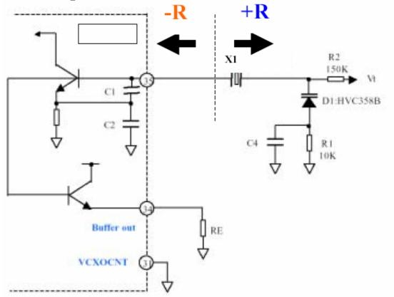
MT6139 procides a VCXO function. With that function, we can build a reference clock generation circuits as shown in the above graph. This means that the VCTCXO module is not necessary for clock application. And only one crystal with 8ppm tolerance and one varactor are enough.
