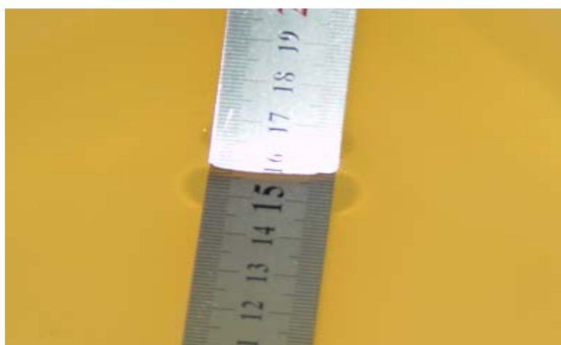
Liquid depth for SAR Measurement
