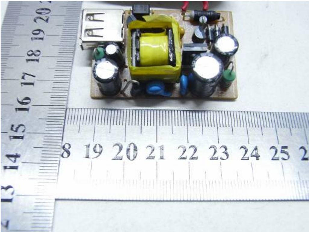
INTERNAL PHOTO OF POWER SUPPLY-1
