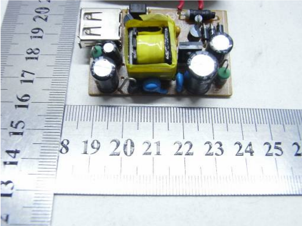
INTERNAL PHOTO OF POWER SUPPLY-1
