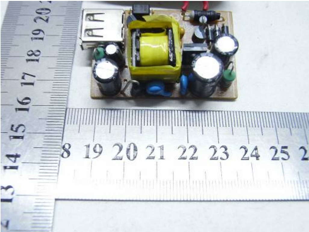
INTERNAL PHOTO OF POWER SUPPLY-1
