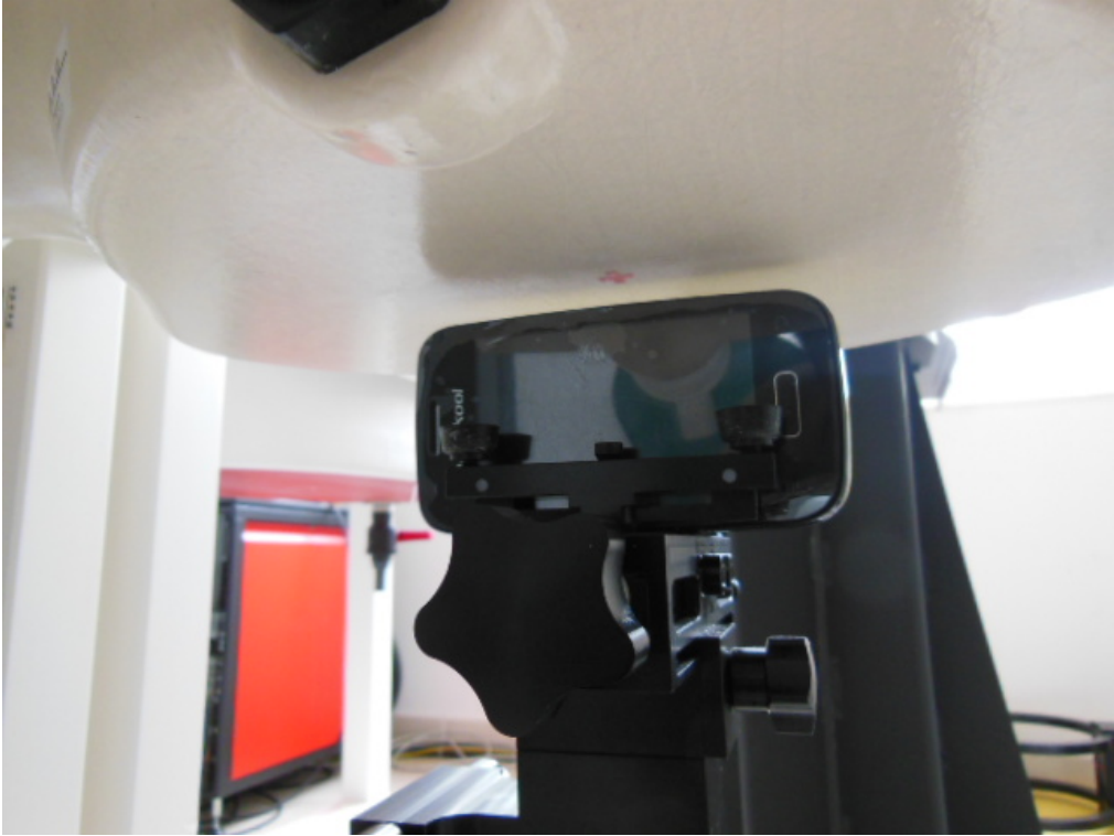
10mm Body-worn Right Side Setup Photo
