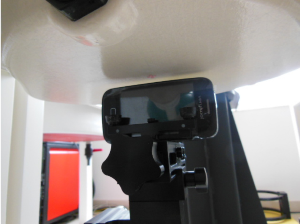
10mm Body-worn Left Side Setup Photo
