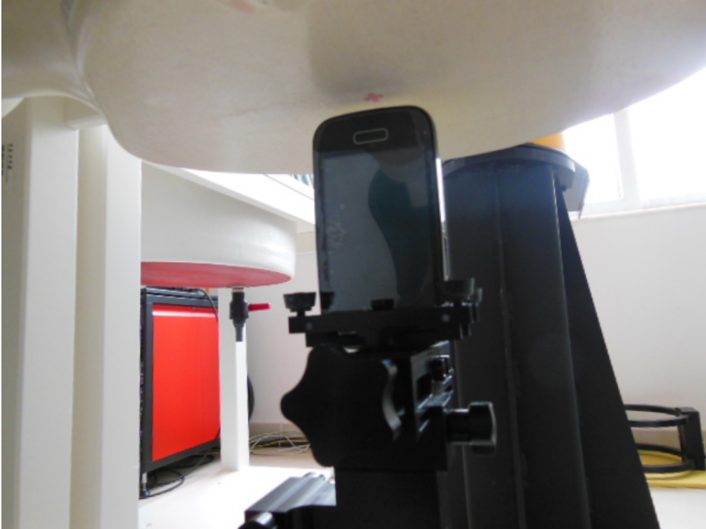
10mm Body-worn Bottom Side Setup Photo
