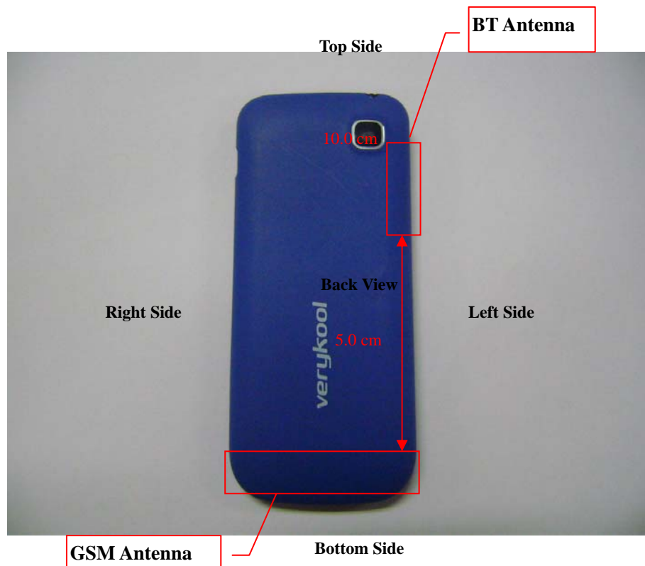
Fig 7.5 Block Diagram for EUT Antenna Position
