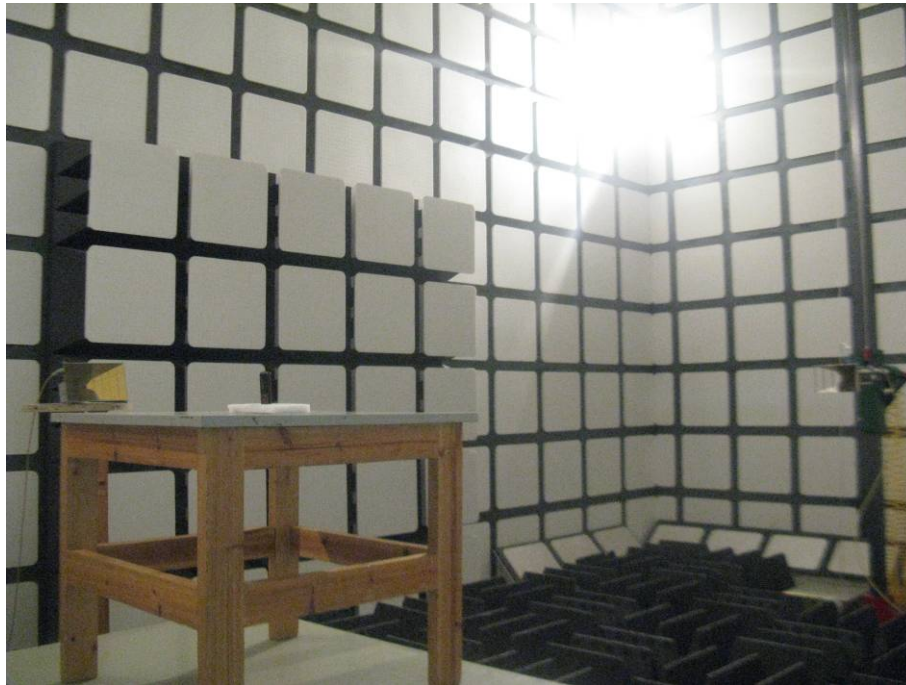
Above 1GHz: Radiated Emissions - Front View
