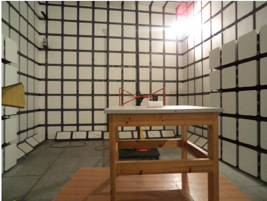
Below 1GHz: Radiated Emissions - Front View
