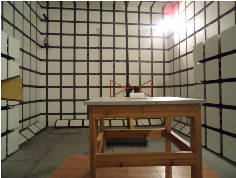
Below 1GHz: Radiated Emissions - Rear View
