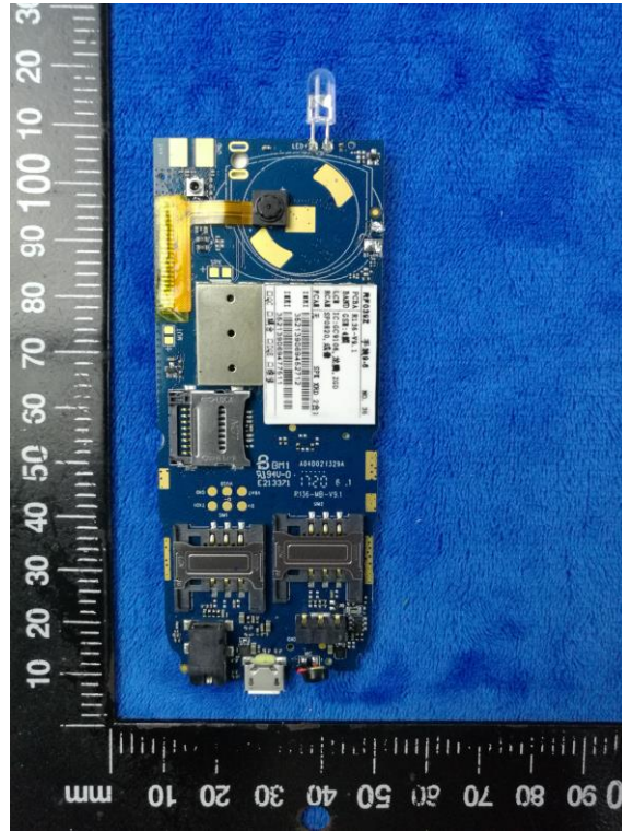
Mainboard with Shielding – Front View
