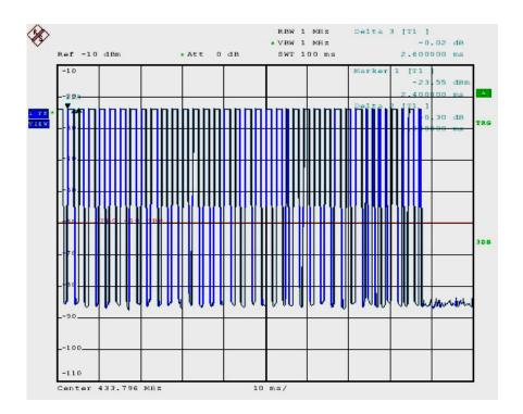
The above graph shows the duration of "on" signal, duration time = 88 ms During the data transmission, we find that data transmitted also periodically. It sends data 1.6ms, and then be silent 1ms, and continue to send data, so the duty cycle =  $[1.6ms / (1.6ms + 1ms) \times 88ms] / 100ms = 54.15\%$
