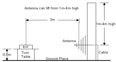
EUT: Wireless Weather Station (Transmitter)
