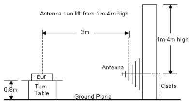
EUT: Wireless Weather Station (Transmitter)
