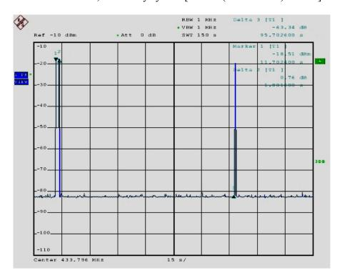
The above graph shows the silent period of "off" signal, silent period is 95.7s. The above graph shows the transmissions are sent at periodic rate automatically.
