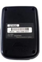
The ST690 with its holderis a waterproof (IP66compliant) hard-cased ultra-mini tracking device to be used for various purposes like an asset tracker or a personal tracker.
