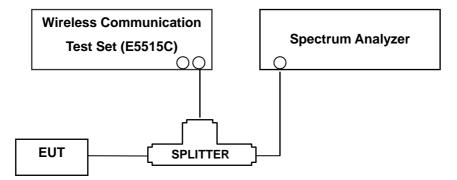
(Configuration of conducted Emission measurement)
