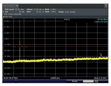
GSM850 MODE (128 CH.) Conducted Spurious Emissions1
