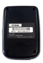
The ST4940 with its holderis a waterproof (IP66compliant) hard-cased ultra-mini tracking device to be used for various purposes like an asset tracker or a personal tracker.
