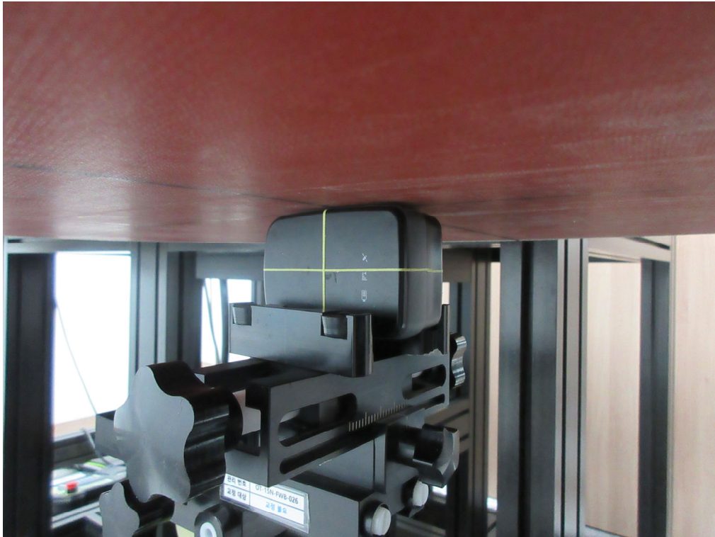
Left from Flat Phantom (Separation Distance: 0 cm)
