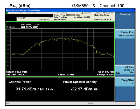
PAPR (dB) = P<sub>Pk</sub> (dBm) - P<sub>Avg</sub> (dBm) = 32.11 dBm - 31.71 dBm = 0.4 dB
