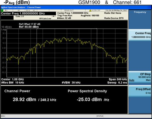
PAPR (dB) = P<sub>Pk</sub> (dBm) - P<sub>Avg</sub> (dBm) = 29.30 dBm - 28.92 dBm = 0.38 dB
