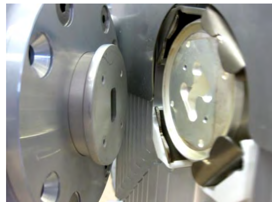
Example of horizontal polarization interconnection
