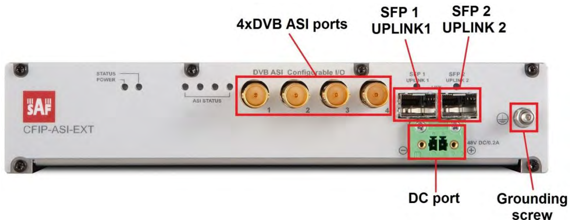
Figure 1.15 ASI EMM extension module interfaces
