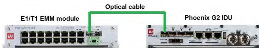
Figure 1.26 Phoenix G2 IDU and E1/T1 EMM module interconnection
