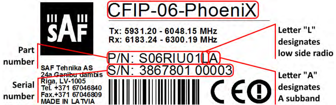
Figure 1.6 Label of the Phoenix G2 IRFU
