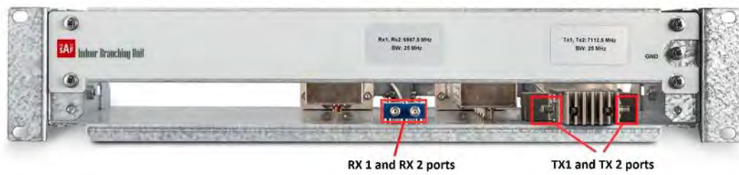
Figure 1.42 IBU front panel interfaces
