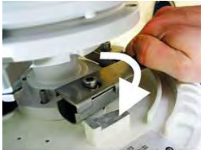
Figure 2.3 Locking of ODU with tightening tool
