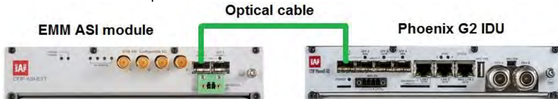
Figure 1.16 Phoenix G2 IDU and ASI EMM module interconnection
