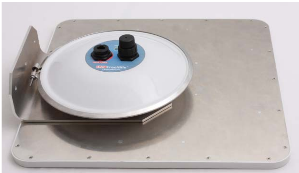
Figure 5 – FreeMile 5.8GHz MIMO with integrated antenna
