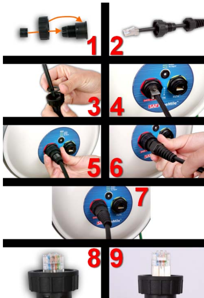
Figure 5. Assembling Ethernet weatherproof connector
