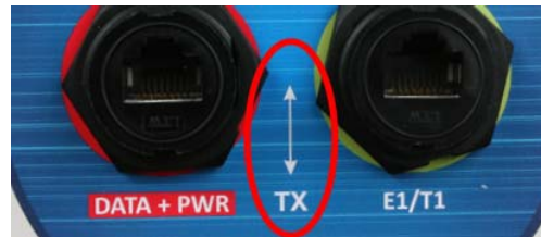
Figure 3. SAF FreeMile set to vertical polarization
