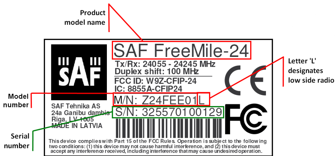
Figure 2. Label of the SAF FREEMILE-24 FODU Low band side
