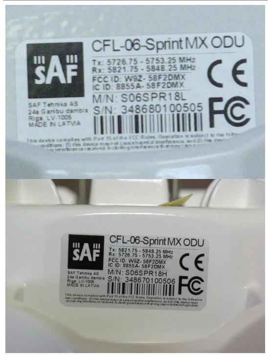
Rogers Labs, Inc. 4405 W. 259th Terrace Louisburg, KS 66053 Phone/Fax: (913) 837-3214 Revision 1 SAF Tehnika AS S/N's: 348 Models: S06SPR18L and S06SPR18H Test #: 170615 Test to: 47CFR, 15.407, RSS-247 File: 58F2DMX LabelSmpl
