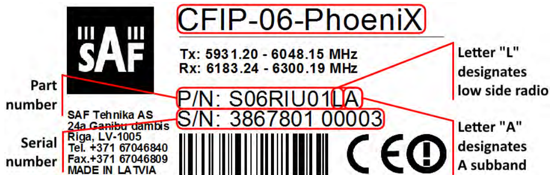
Figure 1.13 Label of the CFIP Phoenix IRFU Low band side, operating in 6 GHz band
