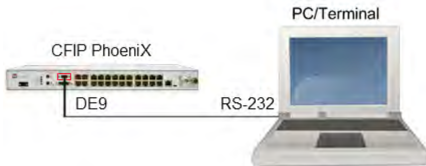
Figure 2.14 Serial connection to CFIP Phoenix
