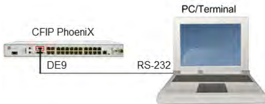
Figure 2.14 Serial connection to CFIP Phoenix
