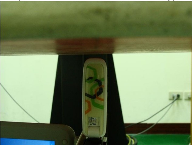
Direct Laptop Plug-in for USB Configuration 5 (Tip Mode with Phantom 0.5 cm Gap)
