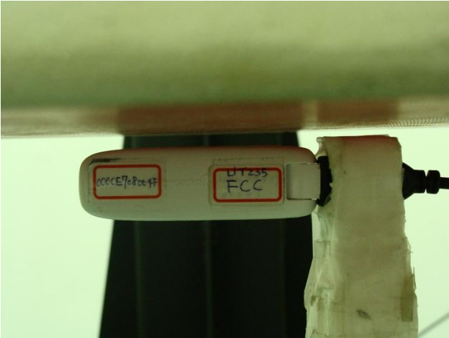
USB Cable Plug-in for USB Configuration 3 (Vertical Front with Phantom 0.5 cm Gap)
