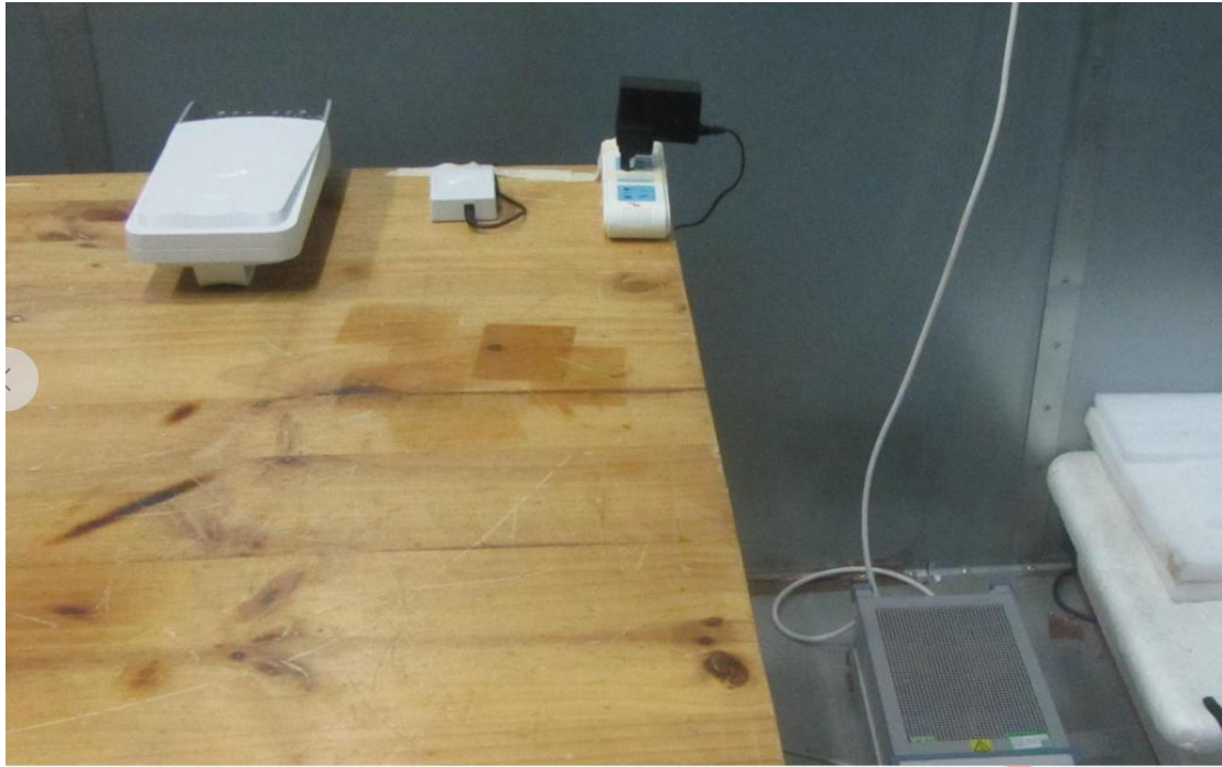
Picture 3 Conducted Emission Test Setup
