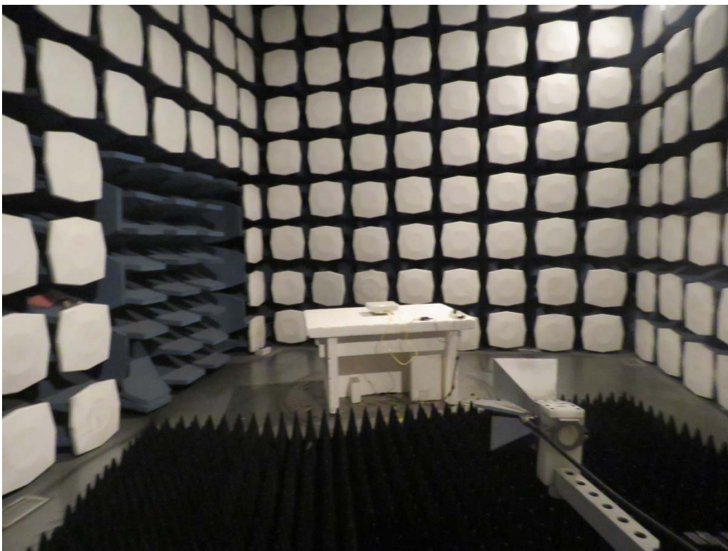
Picture 2: Radiated Spurious Emissions Test setup
