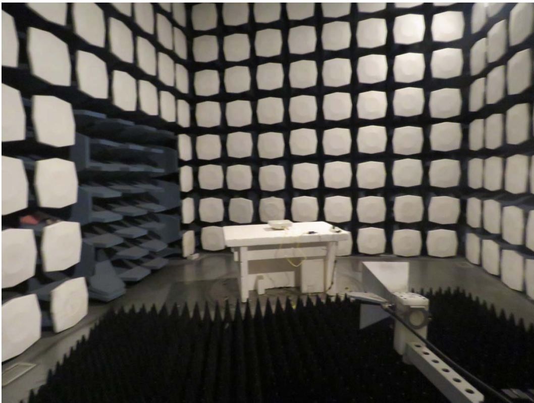
Picture 2: Radiated Spurious Emissions Test setup
