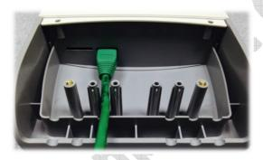
Connect PC to WN-200 or PoE injector for configuring Outdoor CPE Device: Connect WN-200's LAN, or PoE injector's LAN port, to computer by using the device cable.
