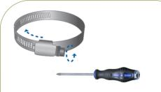
**Step 1** Loosen the locking mechanism of metal strap by hand or screwdriver
