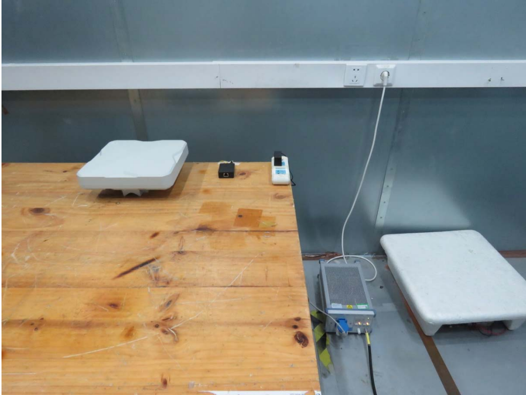
Picture 2 Conducted Emission Test Setup
