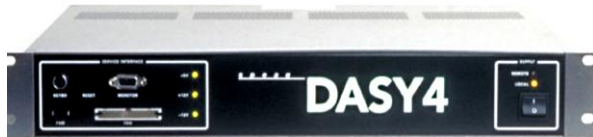
Fig 5.7 Photo of Server for DASY4
