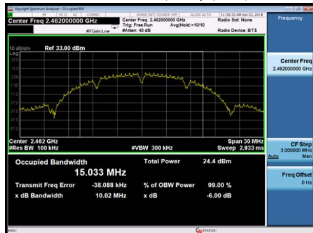
802.11b, Carrier frequency (MHz): 2462
