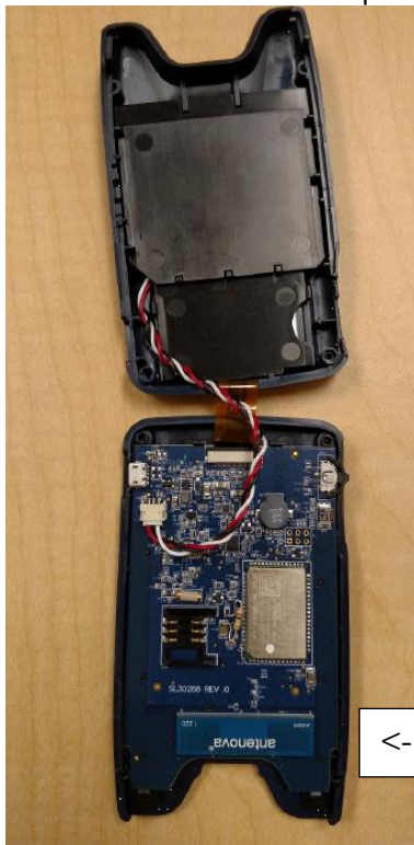
Picture 1: Device with the top cover lifted showing the cellular antenna.
