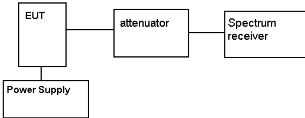
**Method of Measurement:** The procedure used was ANSI/TIA-603-C: 2004 or ANSI 63.4:2003
