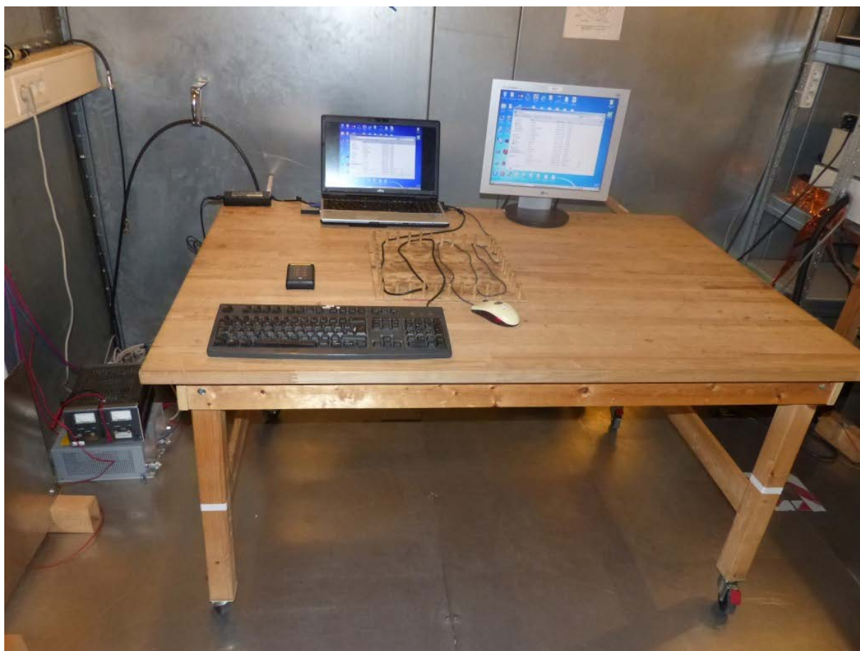
Photo 4: Test setup for conducted measurements (AC/DC adapter, 120 V/60 Hz, EMC insulated room, unintentional radiator, § 15)
