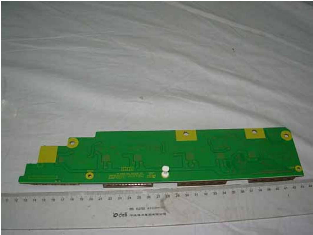
FIGURE 21 PDP TV (M/N: ELPCFT501) H.V. BOARD#1 (SOLDERED SIDE)
