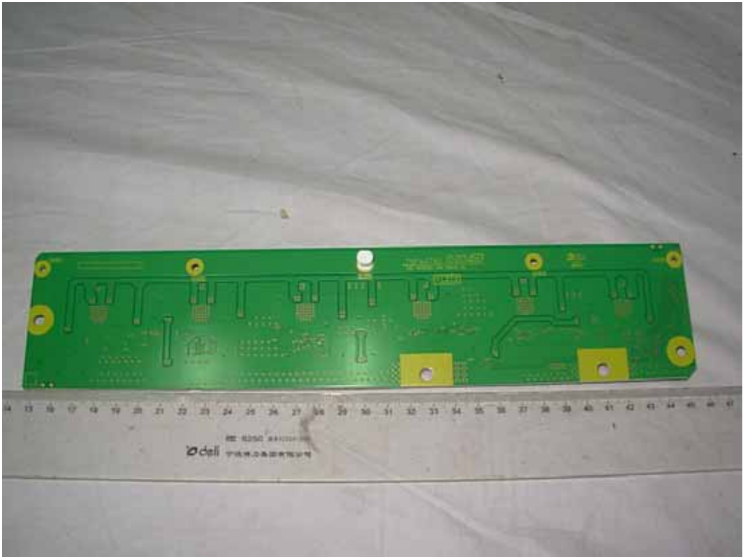
FIGURE 23 PDP TV (M/N: ELPCFT501) H.V. BOARD#2 (SOLDERED SIDE)
