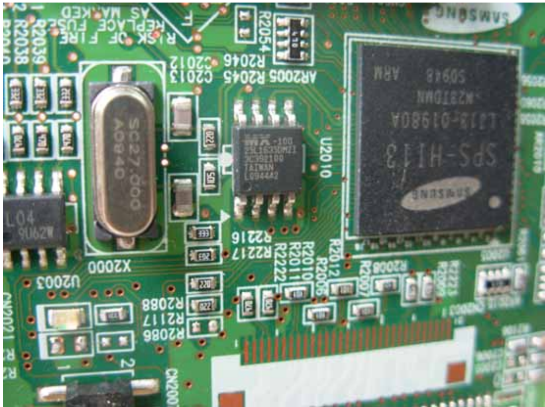
FIGURE 12 LCD TV (M/N: PHDN42M78US) CHIP & CRYSTAL ON DISPLAY BOARD
