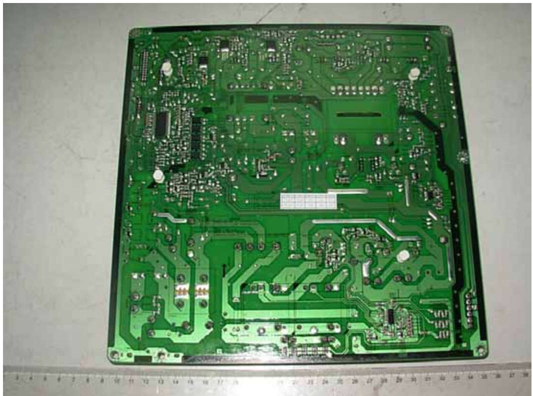
FIGURE 3 LCD TV (M/N: PHDN42M78US) POWER BOARD (SOLDERED SIDE)
