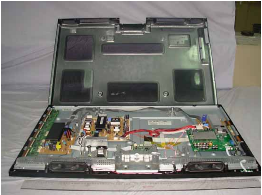
FIGURE 1 LCD TV (M/N: PHDN42M78US) COVER REMOVED
