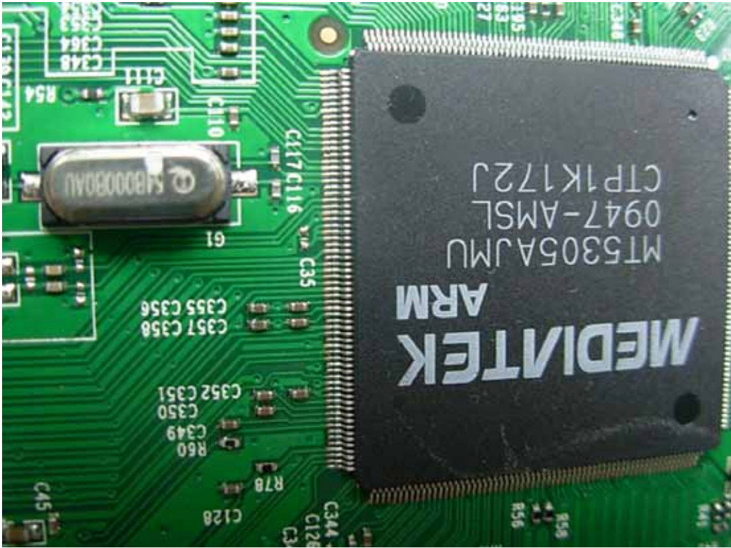
FIGURE 6 LCD TV (M/N: PHDN42M78US) CHIP & CRYSTAL ON MAIN BOARD
