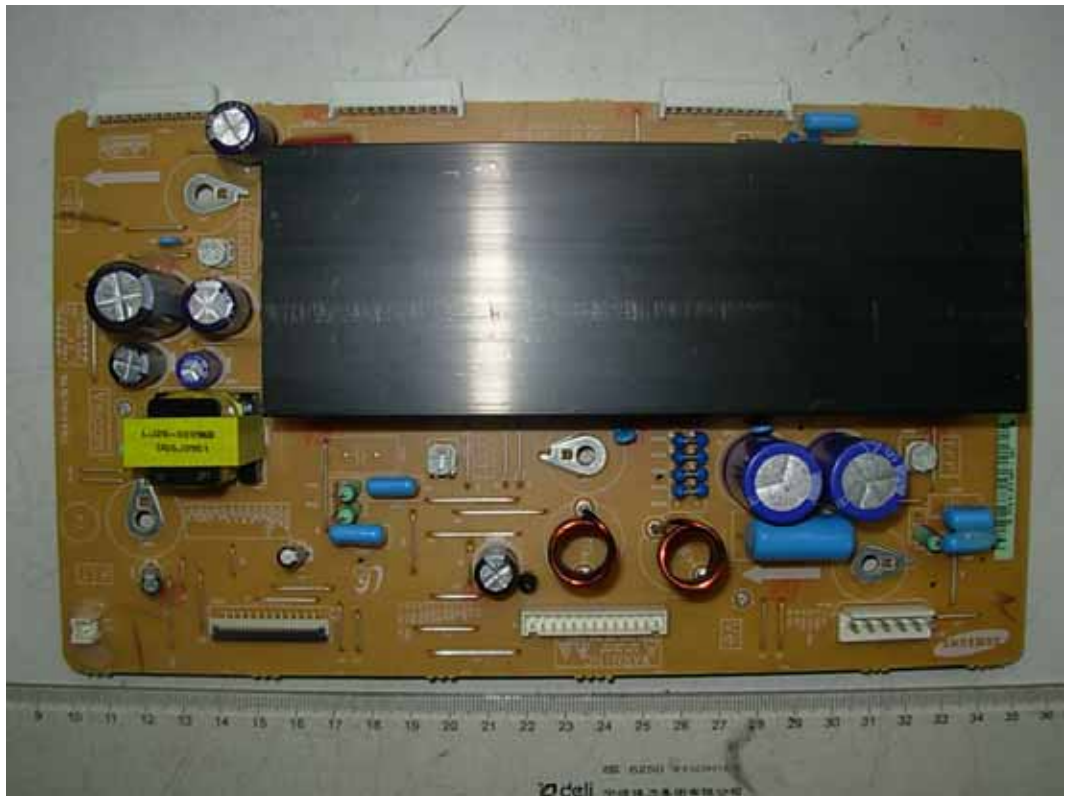
FIGURE 13 LCD TV (M/N: PHDN42M78US) VSCAN BOARD (COMPONENT SIDE)
