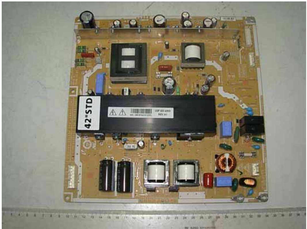
FIGURE 2 LCD TV (M/N: PHDN42M78US) POWER BOARD (COMPONENT SIDE)
