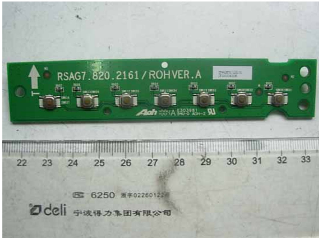
FIGURE 19 LCD TV (M/N: PHDN42M78US) KEY BOARD (COMPONENT SIDE)
