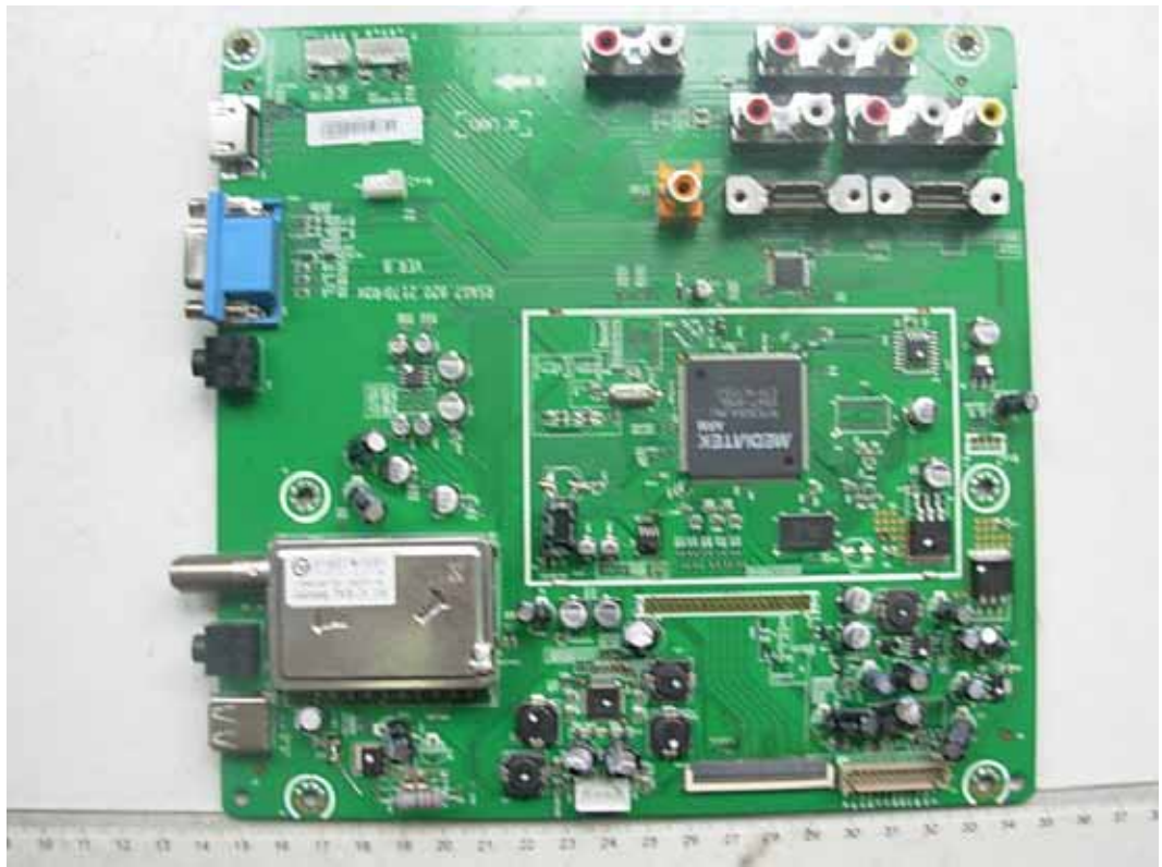
FIGURE 4 LCD TV (M/N: PHDN42M78US) MAIN BOARD (COMPONENT SIDE)
