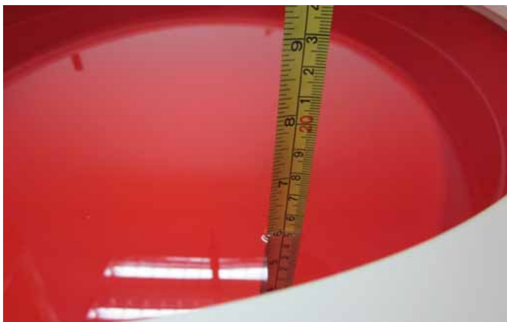
Figure 4.4: Liquid depth in the Flat Phantom
