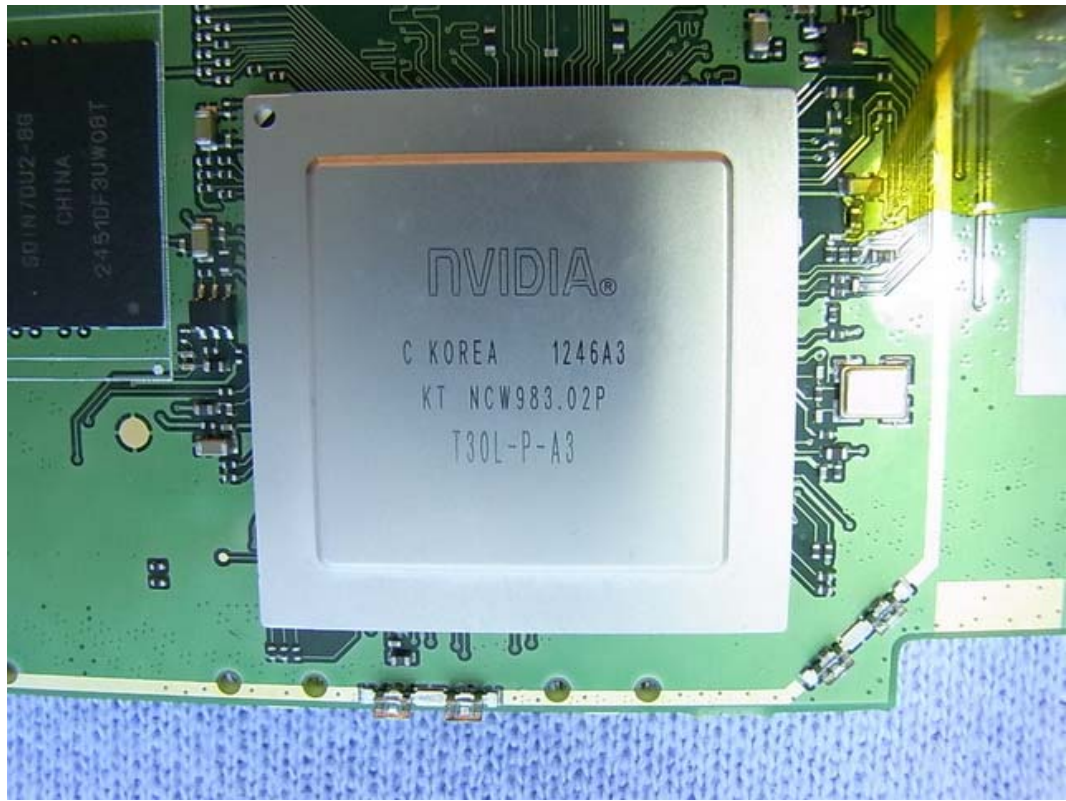
FIGURE 11 SERO 7 PRO (M/N: M470BSA) CPU ON MAIN BOARD
