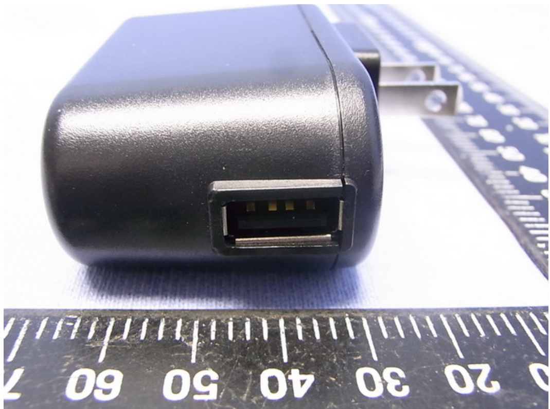
FIGURE 15 SERO 7 PRO (M/N: M470BSA) ADAPTER (USB PORT)
