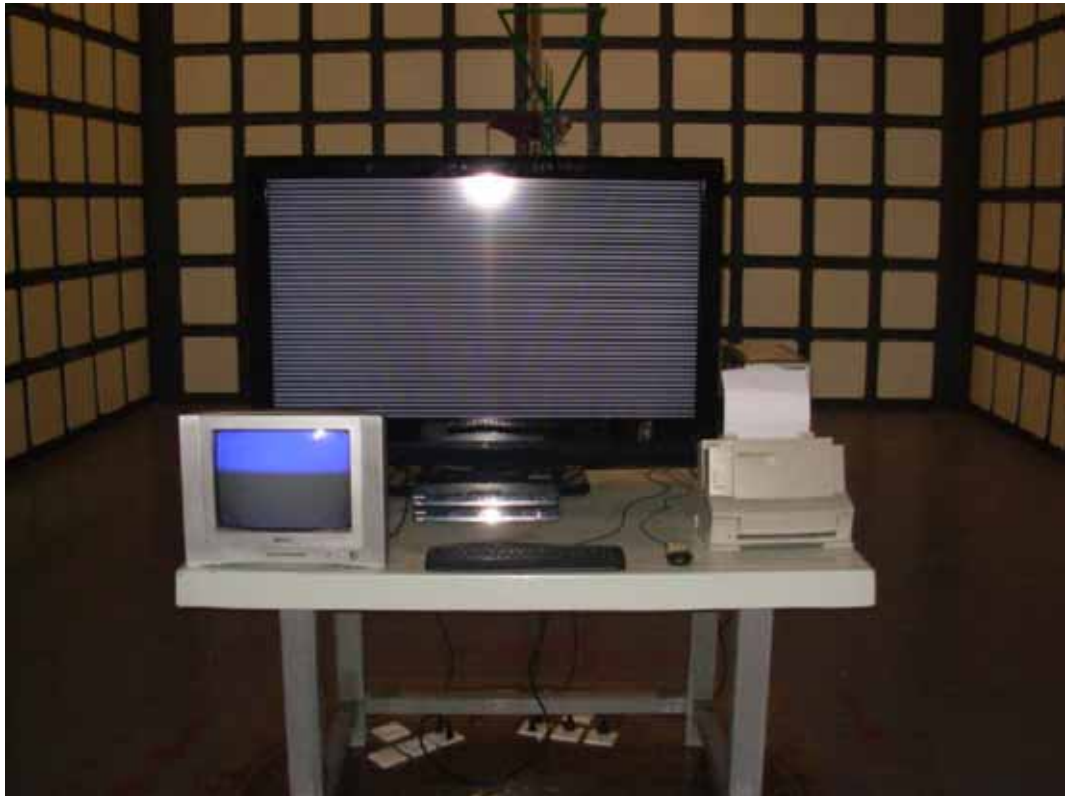
FRONT VIEW OF RADIATED EMISSION TEST
