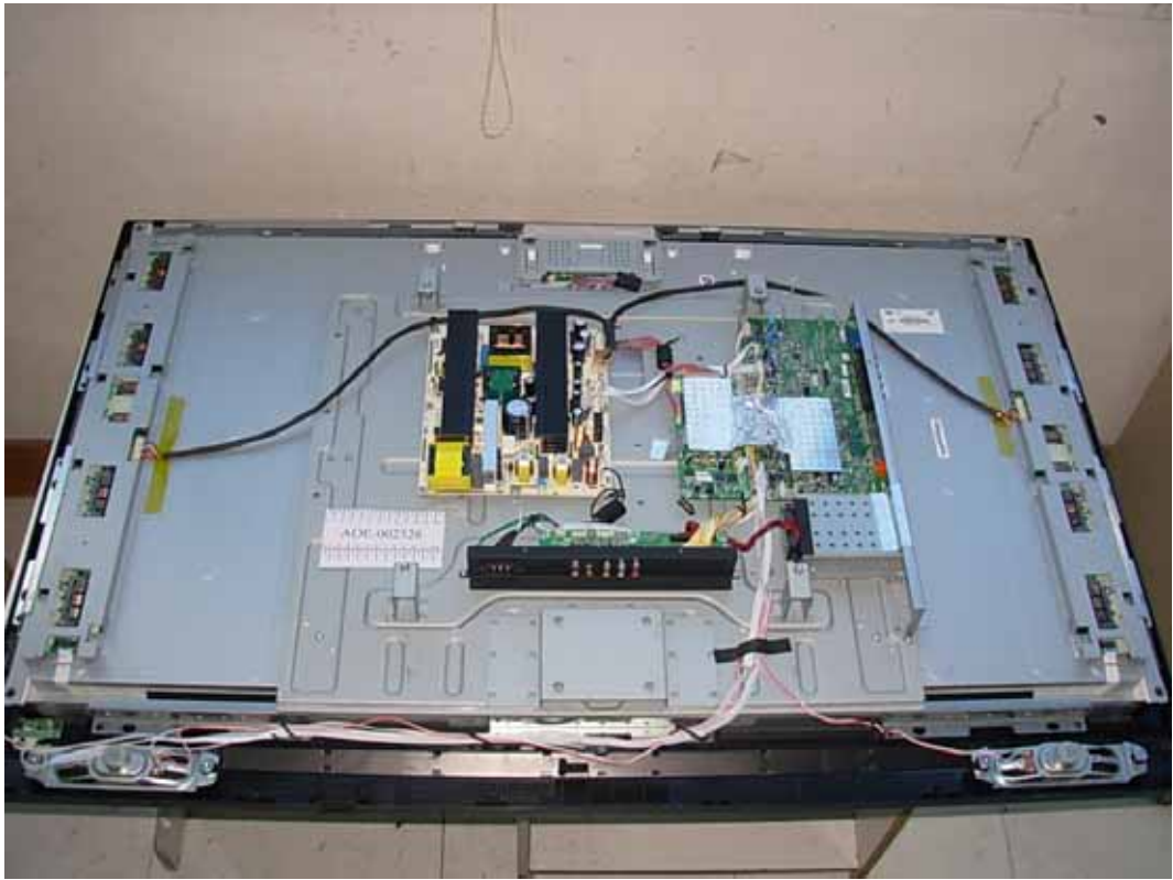
FIGURE 1 LCD MONITOR (M/N: NVU52FX5) COVER REMOVED
