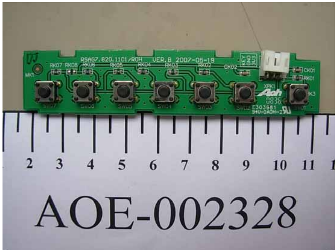
FIGURE 23 LCD MONITOR (M/N: NVU52FX5) BUTTON BOARD (COMPONENT SIDE)
