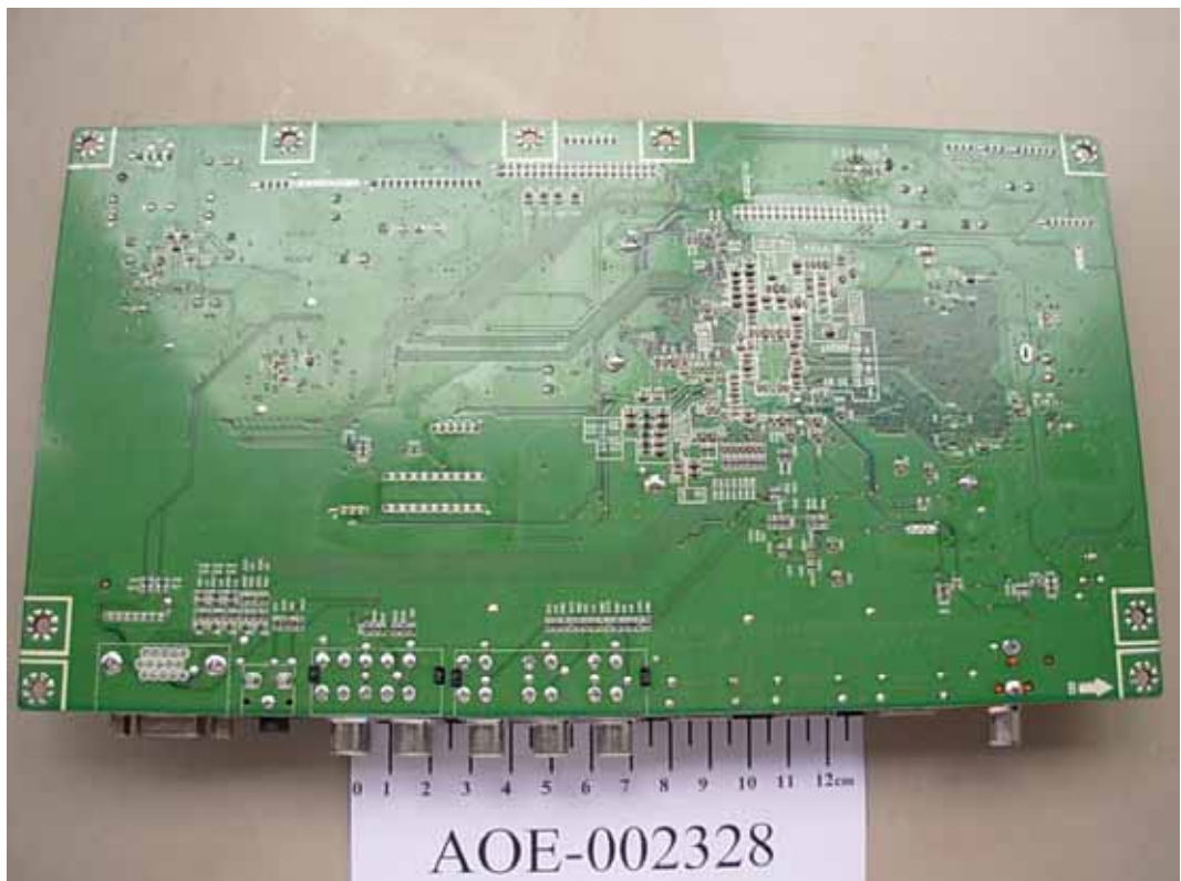
FIGURE 5 LCD MONITOR (M/N: NVU52FX5) MAIN BOARD 1 (SOLDERED SIDE)
