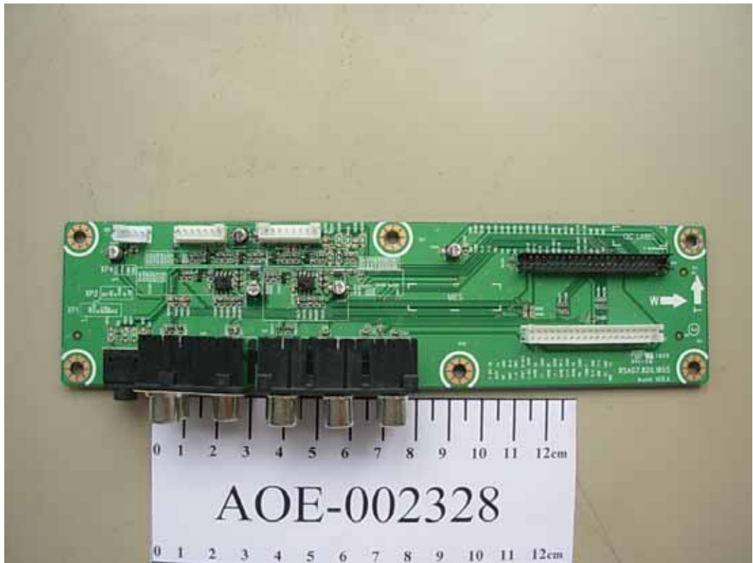
FIGURE 13 LCD MONITOR (M/N: NVU52FX5) SIGNAL BOARD (COMPONENT SIDE)
