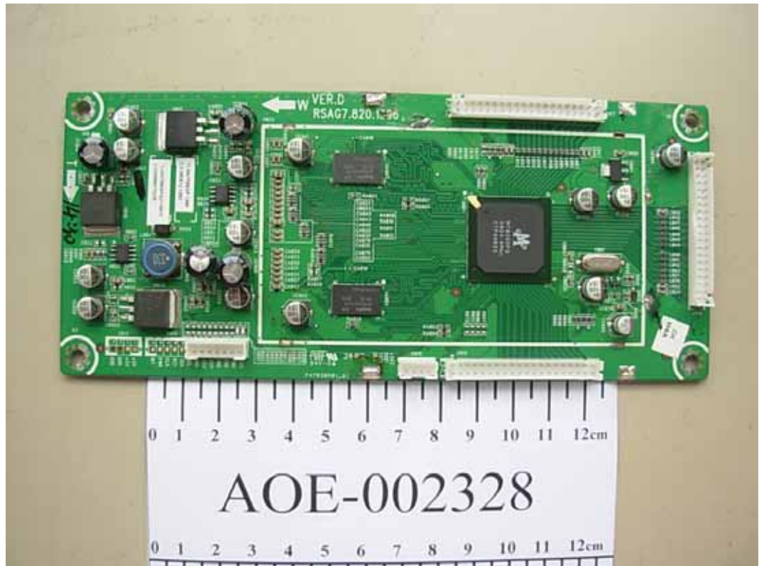
FIGURE 9 LCD MONITOR (M/N: NVU52FX5) MAIN BOARD 2 (COMPONENT SIDE)
