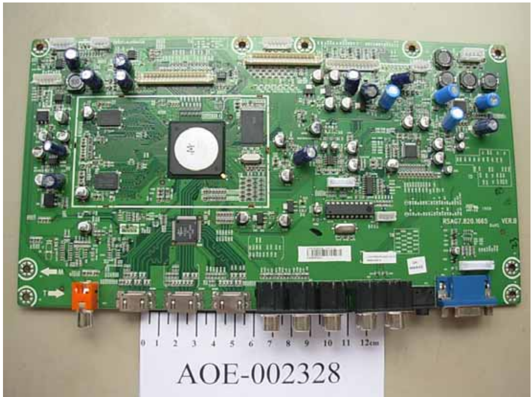
FIGURE 4 LCD MONITOR (M/N: NVU52FX5) MAIN BOARD 1 (COMPONENT SIDE)
