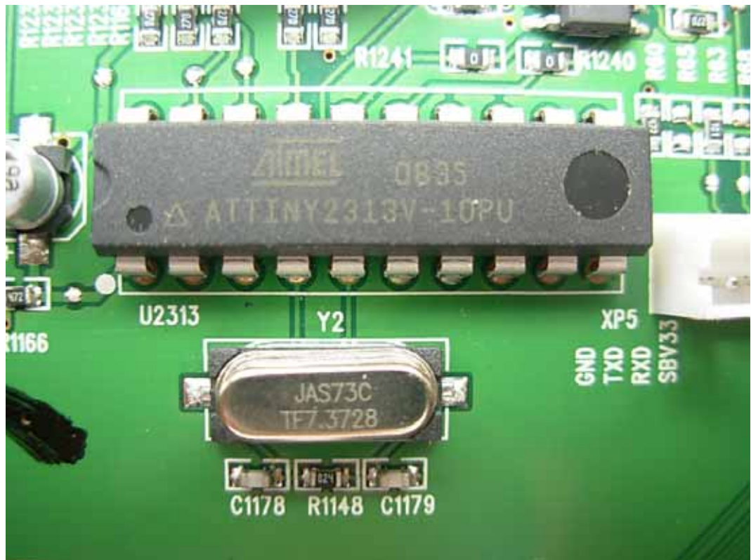
FIGURE 8 LCD MONITOR (M/N: NVU52FX5) CHIP #2 & CRYSTAL #2
