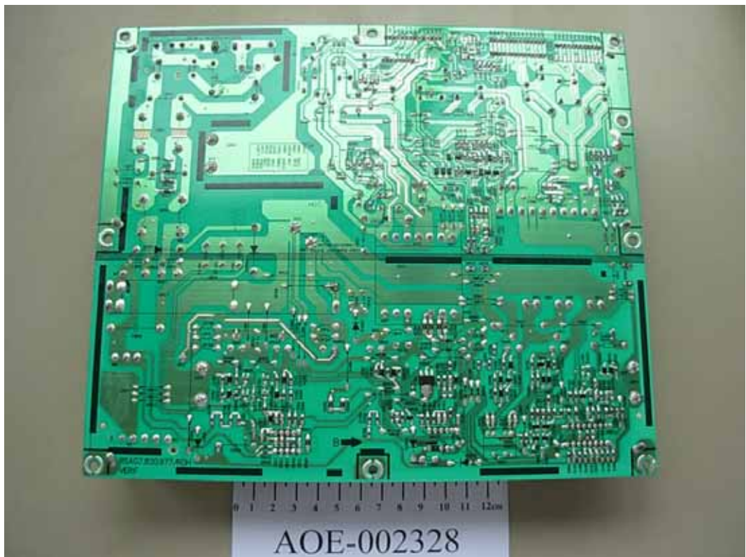
FIGURE 3 LCD MONITOR (M/N: NVU52FX5) POWER BOARD (SOLDERED SIDE)
