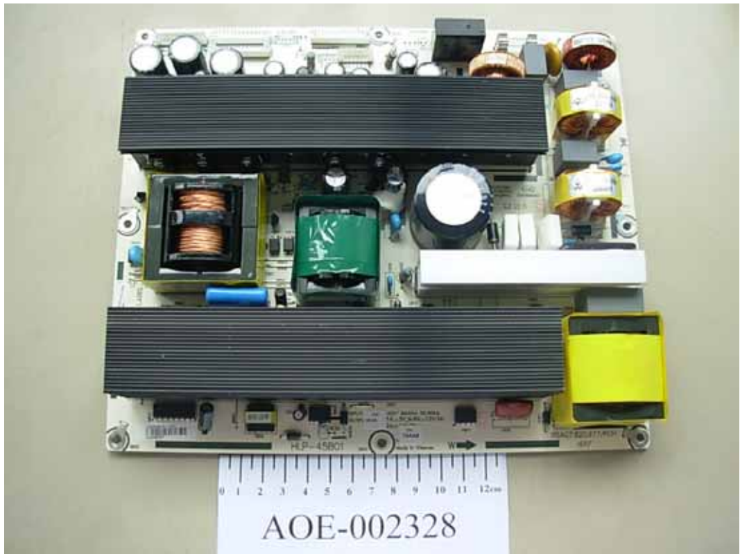
FIGURE 2 LCD MONITOR (M/N: NVU52FX5) POWER BOARD (COMPONENT SIDE)
