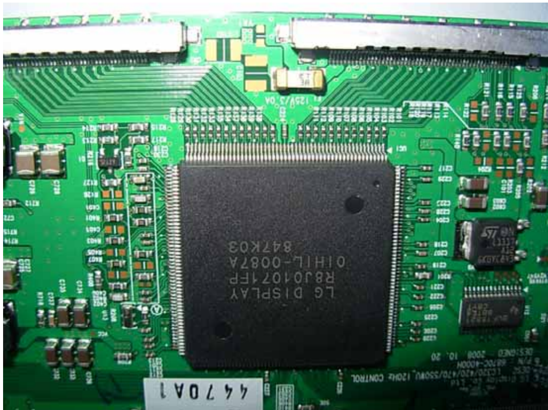
FIGURE 24 LCD MONITOR (M/N: NVU47FX5) CHIP ON PANEL BOARD
