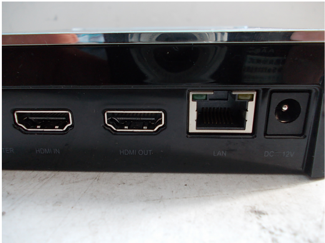
FIGURE 3 NETWORK MEDIA PLAYER (M/N: GX1200V) PORTS #1
