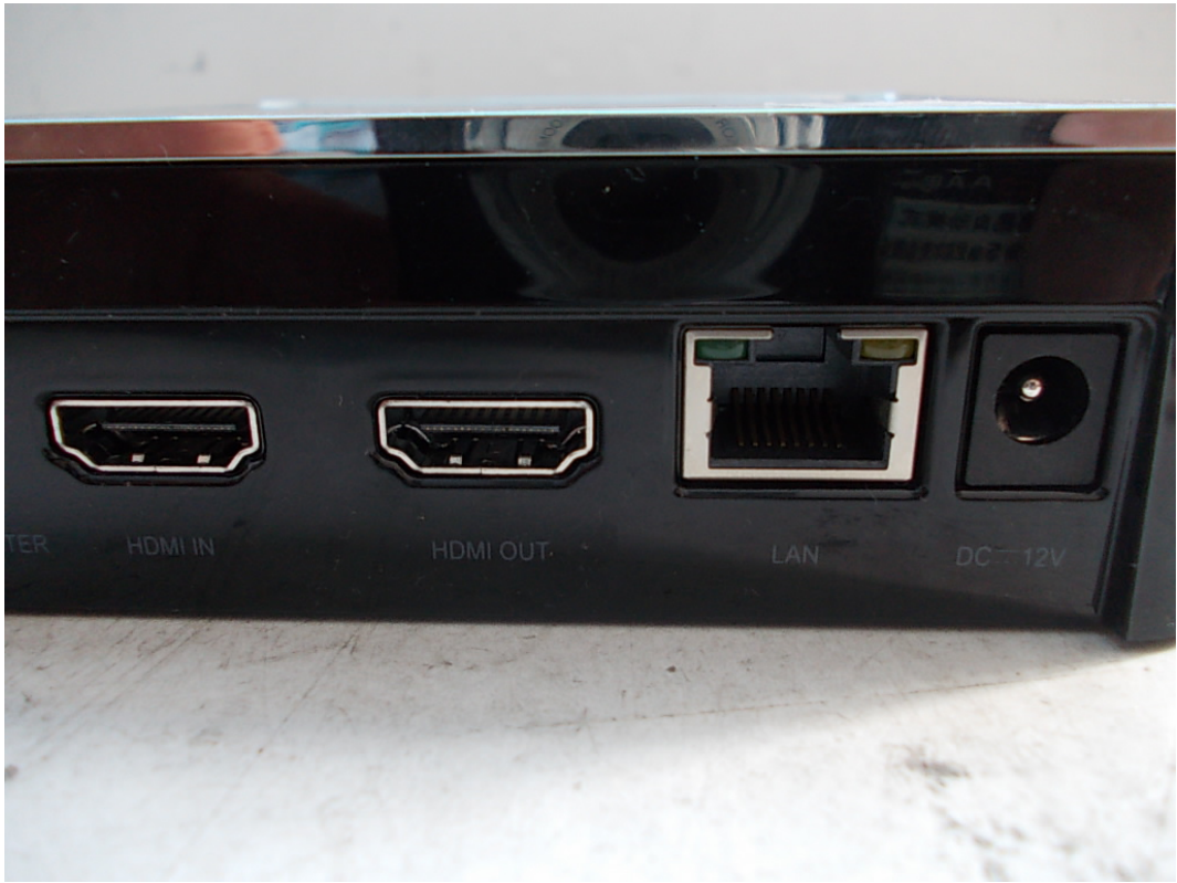
FIGURE 3 NETWORK MEDIA PLAYER (M/N: GX1200V) PORTS #1
