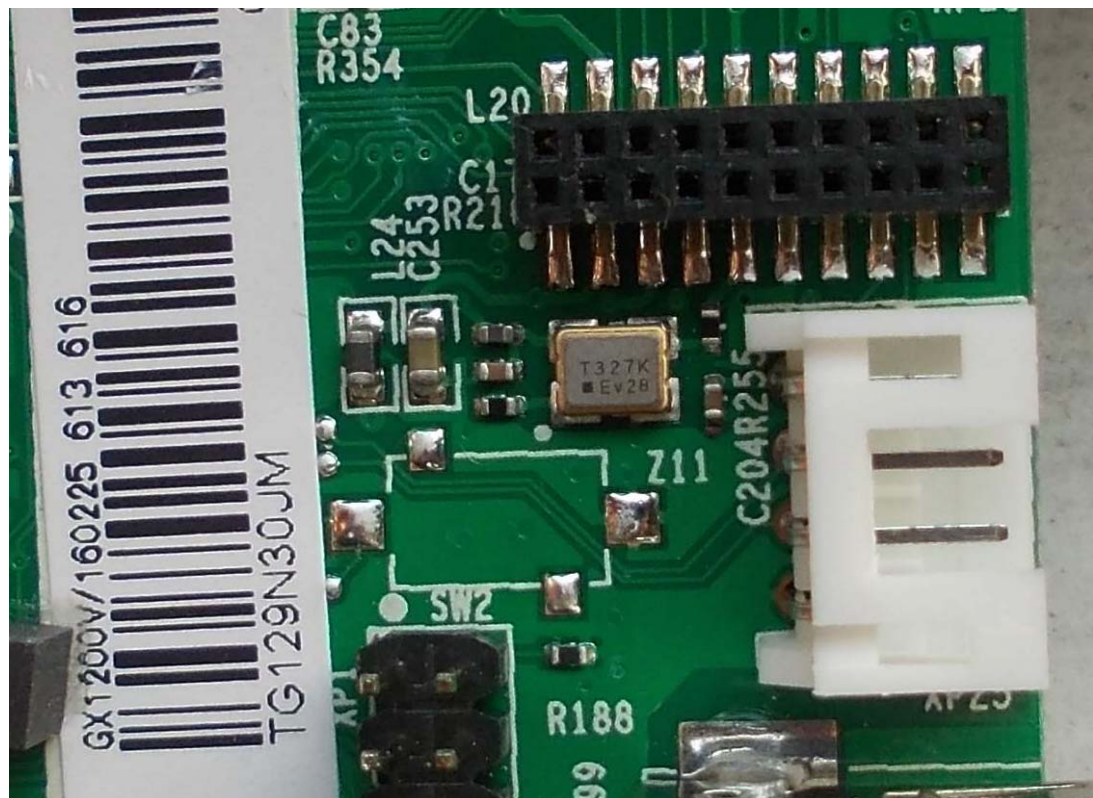
FIGURE 9 NETWORK MEDIA PLAYER (M/N: GX1200V) CRYSTAL #2 ON MAIN BOARD
