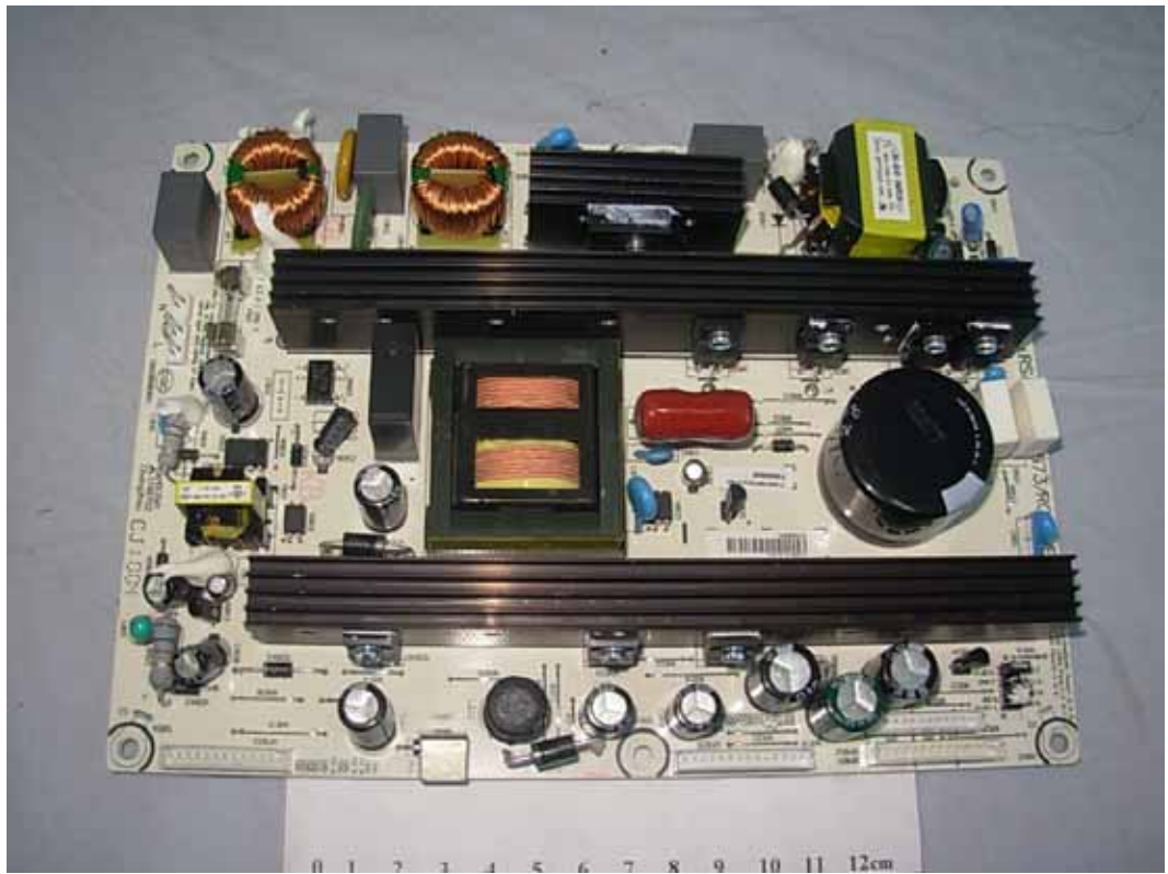
FIGURE 2 LCD TV (M/N: ELCHW402) POWER BOARD (COMPONENT SIDE)
