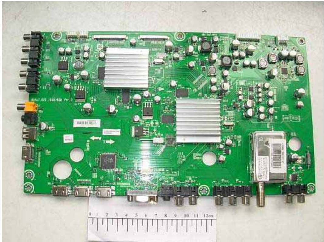
FIGURE 2 LCD TV (M/N: 55LED55SA) MAIN BOARD (COMPONENT SIDE)
