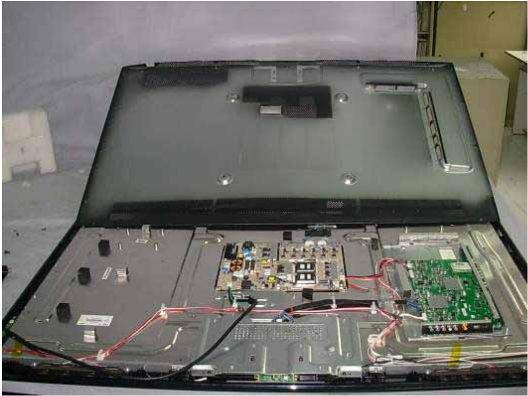
FIGURE 1 LCD TV (M/N: 55LED55SA) COVER REMOVED
