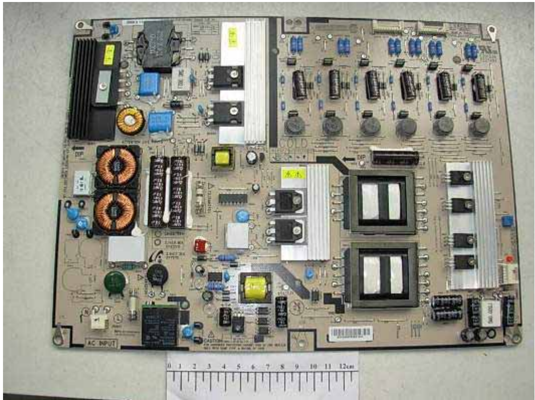
FIGURE 9 LCD TV (M/N: 55LED55SA) POWER BOARD (COMPONENT SIDE)
