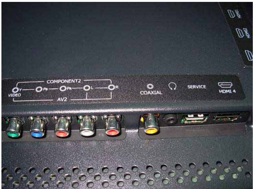
FIGURE 4 LCD TV (M/N: 55LED55SA) BOTTOM PORTS
