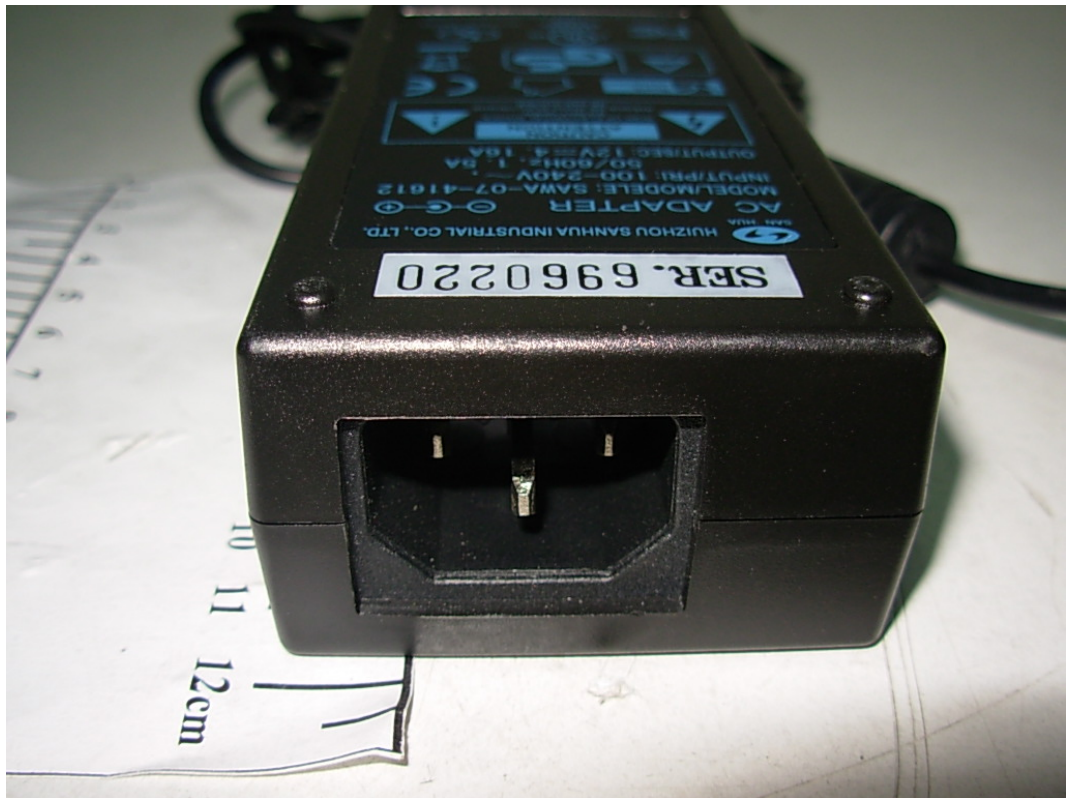
FIGURE 19 LCD TV/DVD COMBO (M/N: LCD19W57DCA) ADAPTER AC IN PORT
