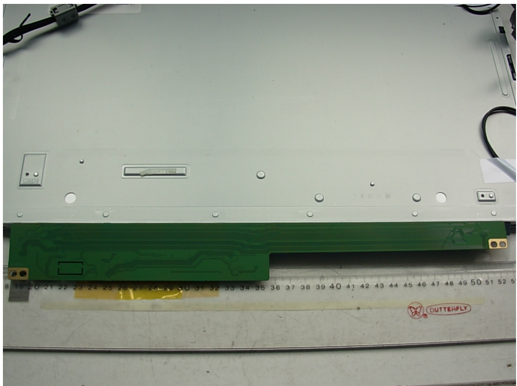
FIGURE 13 LCD TV/DVD COMBO (M/N: LCD19W57DCA) DISPLAY BOARD (SOLDERED SIDE)
