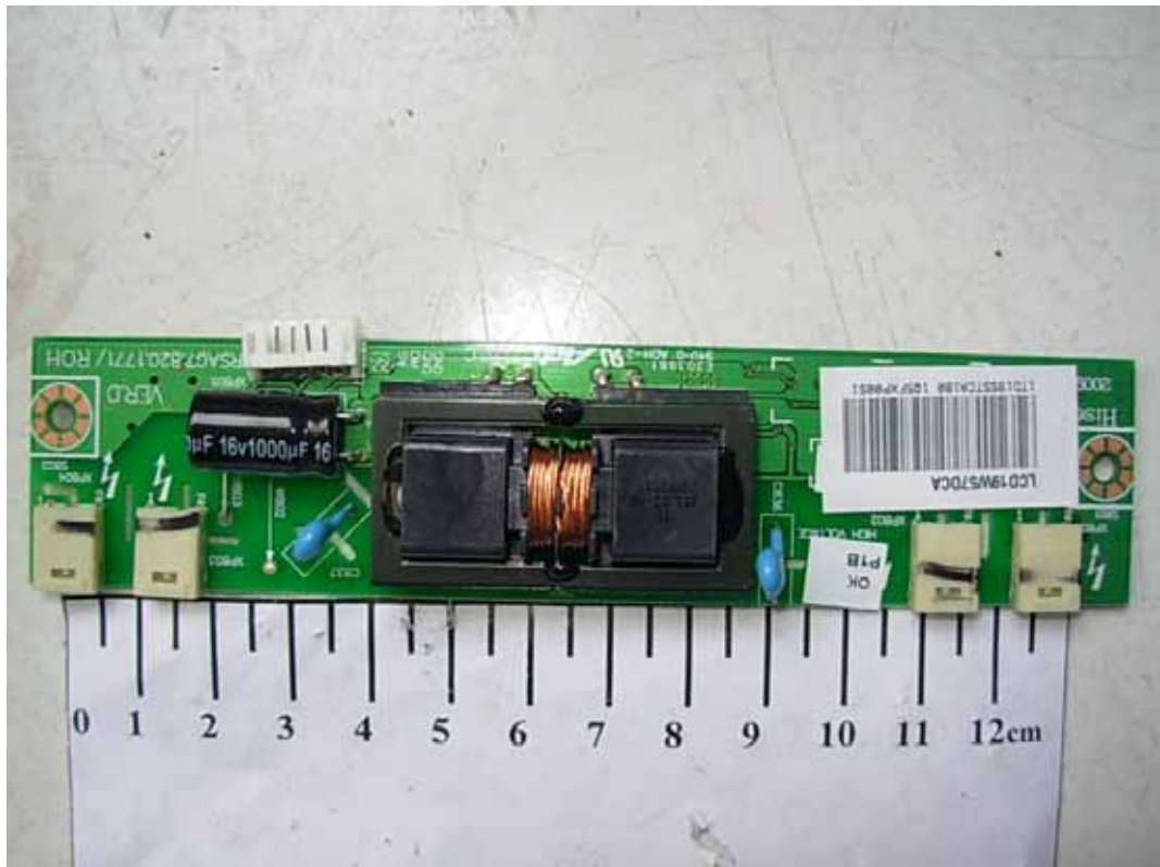
FIGURE 7 LCD TV/DVD COMBO (M/N: LCD19W57DCA) HIGH VOLTAGE BOARD (COMPONENT SIDE)
