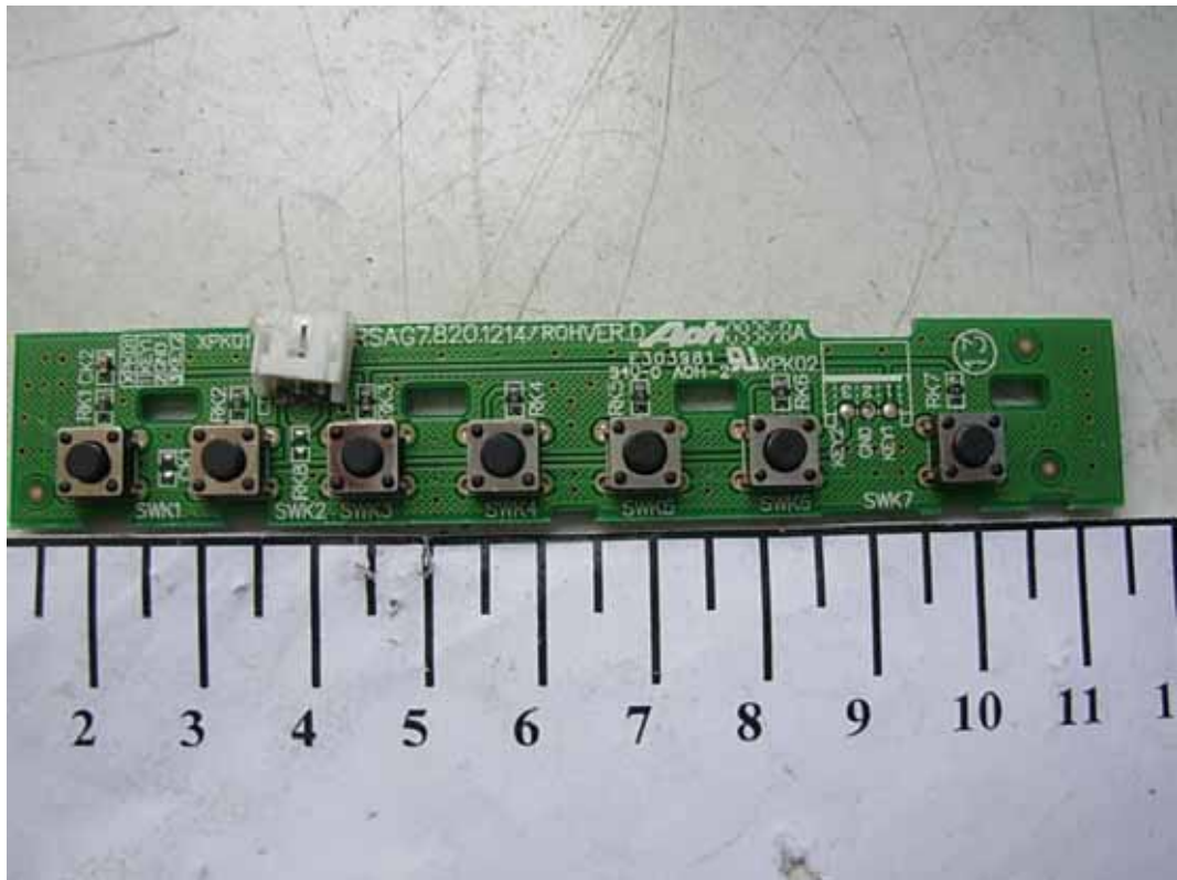
FIGURE 11 LCD TV/DVD COMBO (M/N: LCD19W57DCA) BUTTON BOARD (COMPONENT SIDE)
